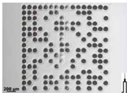
Figure 7: Left – total view of code enlarged 62.5-fold using polarised light microscope, non-analysed transmitted light (PLM/LPNA). Right – 200-fold enlargement of code using SEM/BSE.
