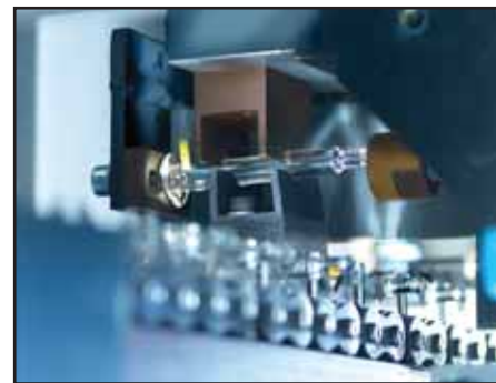
Figure 3: The process of applying the matrix code. A light can be seen at the point of impact of the laser.
