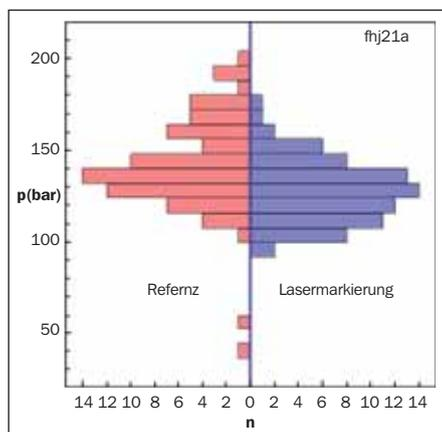
**Figure 6: Double histogram of burst pressure testing.**
