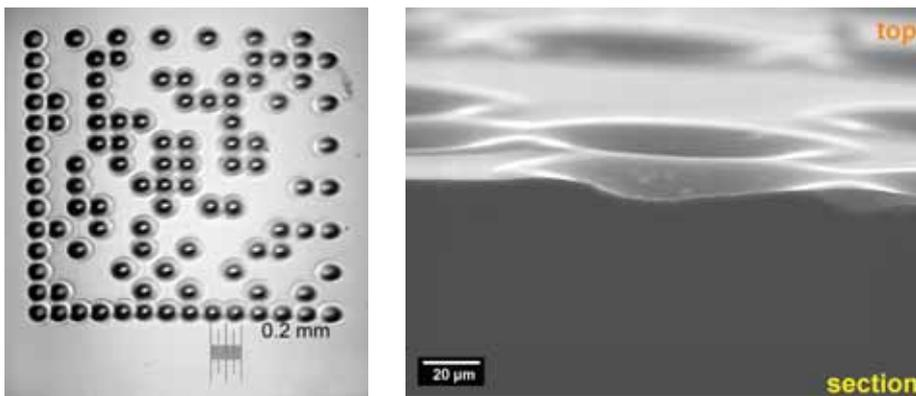
**Figure 1: Left – Matrix code produced by CO<sub>2</sub> laser on heated glass guarantees there are no cracks. Right – SEM/BSE of the cross-section of a code enlarged 700-fold. The intact glass matrix is clearly identifiable.**
