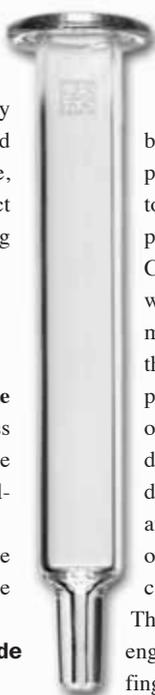
If the transition temperature of the glass is not achieved during the laser process, the syringe is rejected immediately thereafter. This is to ensure that only crack-free, coded material is conveyed further.
