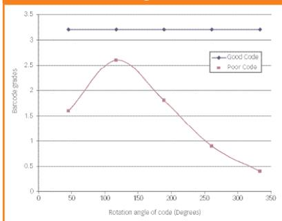
verifier. Why? A macroscopic investigation shows the problem. The code is geometrically distorted, is not symmetrical and therefore does not fit into the reference grid. The lesson learned is straightforward: the human eye cannot replace a specialised measuring instrument.
